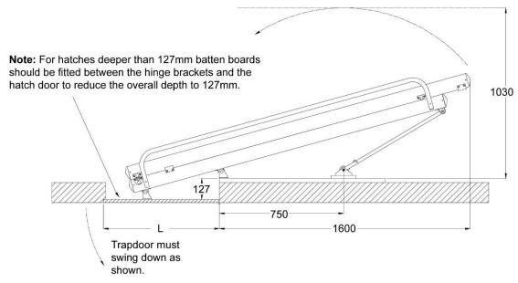
Note: Heavy trapdoors will cause the hatch to remain open.
