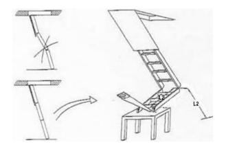
12. Add rubber feet to ladder and nail architrave timber to fit around the ceiling panel to conceal the cut of the opening. Mitre the corners. Fit architrave 2mm
