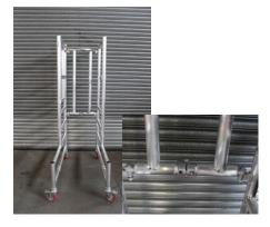
**4.** POSITION CASTORS AT A 45 DEGREE ANGLE AND LOCK IN PLACE.
